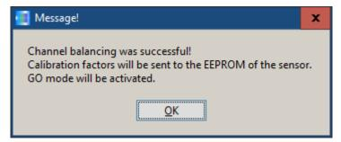
A click on **START SELF CALIBRATION** causes the sensor to calculate the calibration factors itself. It is not possible to specify a **SETVALUE FOR CH0**, **CH1** and a **MAX DELTA OF RAW DATA** here.
