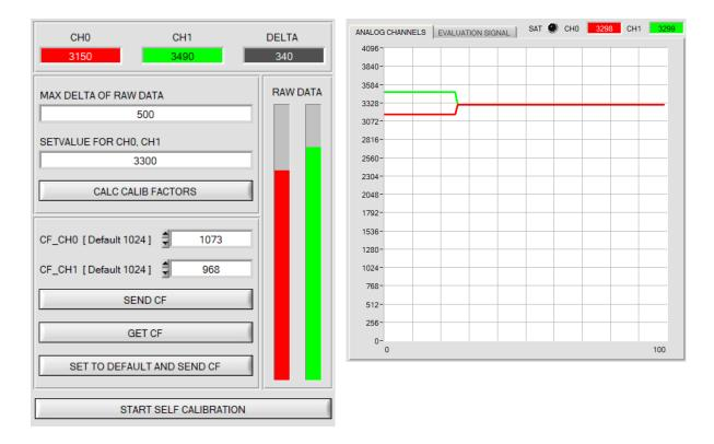
When the calibration factors have been calculated by the software on the user interface, they are automatically saved to the non-volatile **EEPROM** memory of the sensor. Calibration is then finished, work can then be continued in the main panel.
